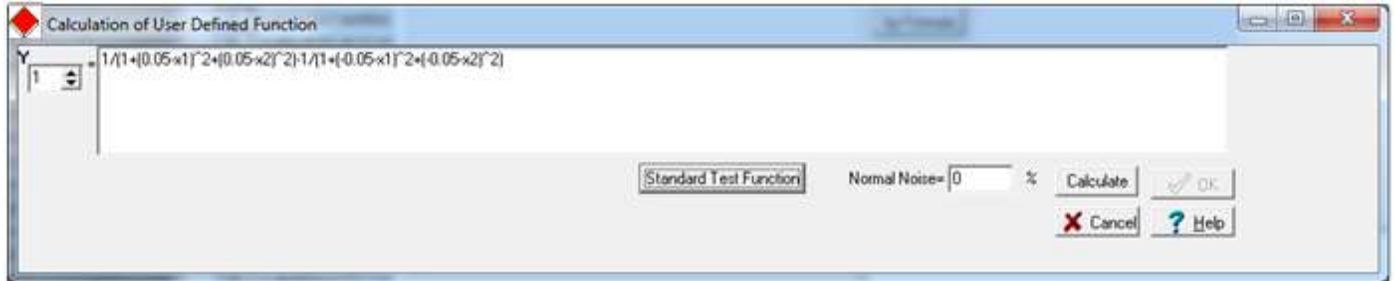
Fig. 23. Entering an analytical function in the response input window
